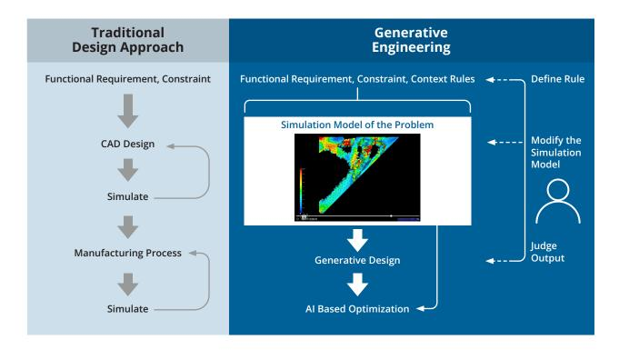
Generative design sees engineers spend far more time and energy outlining constraints **before** the creation of a design. The design is created using algorithms that are informed by these criteria and is then tested through simulation tools and optimized. The different stages of this process are repeated until the engineers are satisfied with the results.
