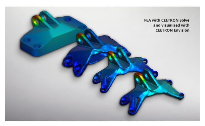
The final image is the result of 57 iterations and is something unlikely to be created through traditional design processes. The designs would then need to be either manually remade in CAD software and machined or be 3D printed as is.
